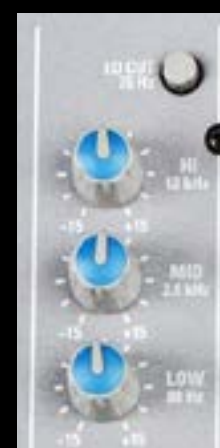
3-band EQ with musical filtering frequencies and LO-CUT
